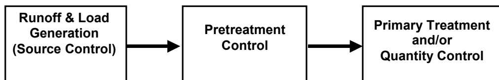
Figure 1.6 Generalized Stormwater Treatment Train
