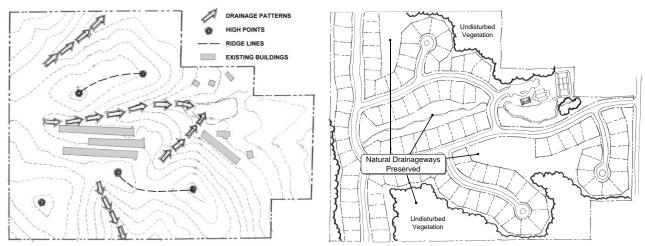
Figure 2.30 Example of a Subdivision Using Natural Drainageways for Stormwater Conveyance and Management
