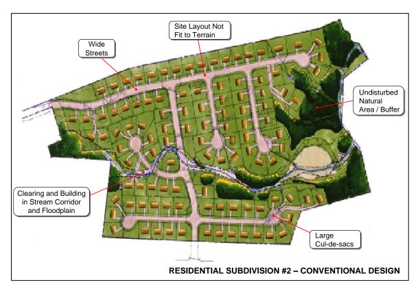
Figure 2.34 Comparison of a Traditional Residential Subdivision Design (above) with an Innovative Site Plan Developed Using *integrated* Site Design Practices (below).
