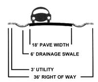
Figure 2.19 Potential Design Options for Narrower Roadway Widths (Source: VPISU, 2000)
