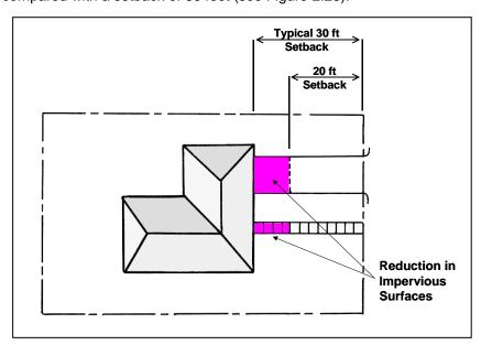
Figure 2.23 Reduced Impervious Cover by Using Smaller Setbacks
