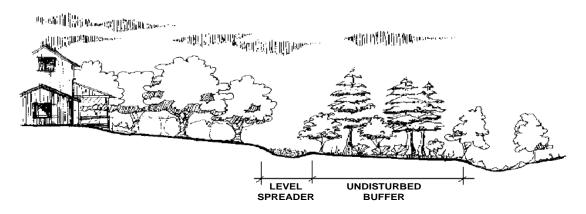
Figure 2.29 Use of a Level Spreader with a Riparian Buffer (Adapted from NCDENR, 1998)
