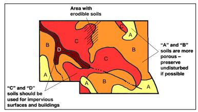
Figure 2.8 Soil Mapping Information Can Be Used to Guide Development
