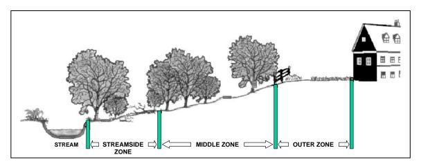
Figure 2.5 Three-Zone Stream Buffer System
