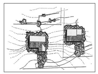
Figure 2.14 Establishing Limits of Clearing (Source: DDNREC, 1997)
