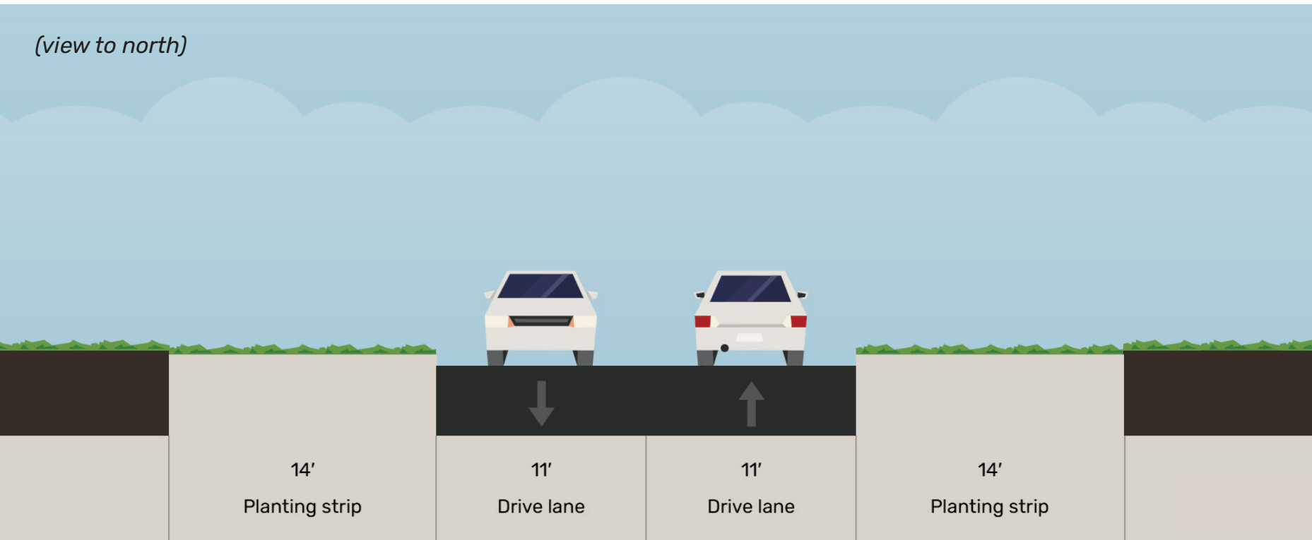
Exhibit 99. Typical Existing Cross-Section on Quail Run Drive (South of Corinth Parkway) (50’ ROW)
