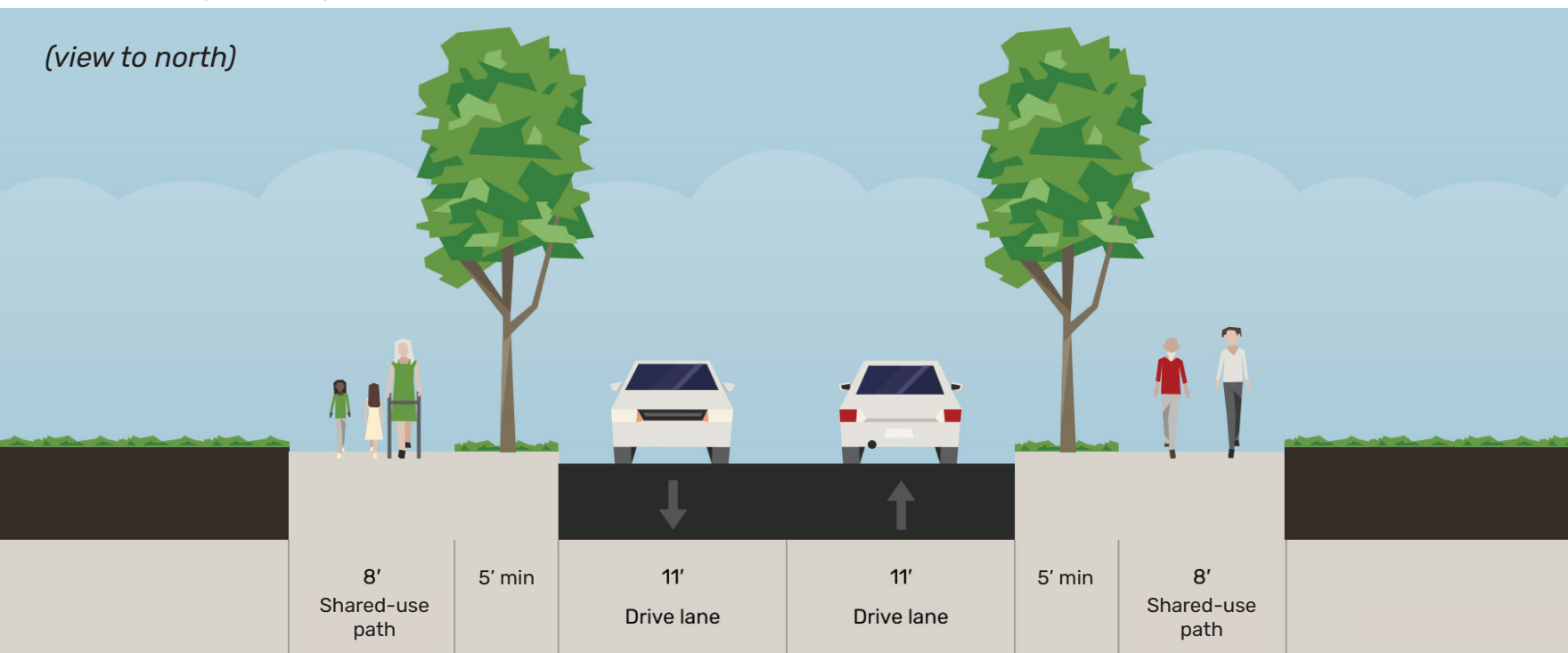
Exhibit 76. Proposed Typical Cross-Section on Garrison Road (North of Cliff Oaks Drive) (60' ROW min)
