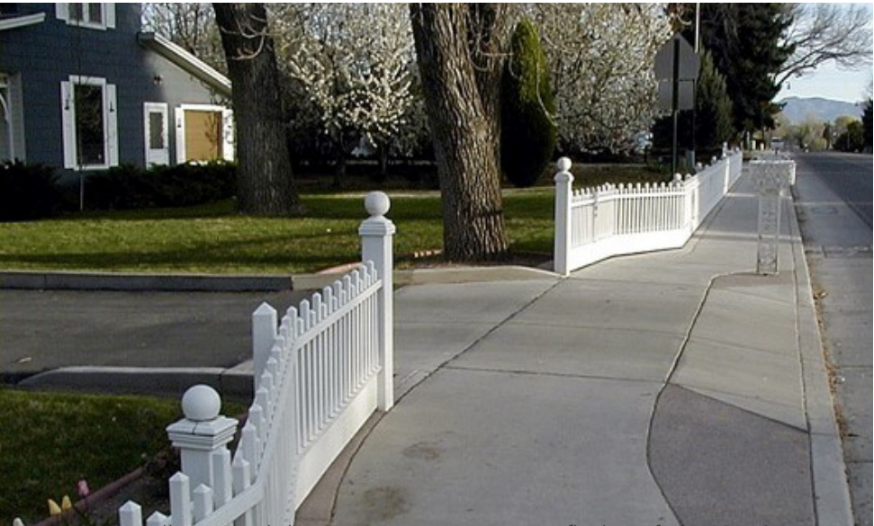
Routing sidewalks around driveway ramps maintain a flush surface. (Credit: Dan Burden)
