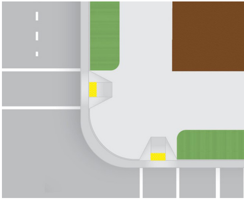
One curb ramp per crosswalk should be provided at corners. Ramps should align with sidewalks and crosswalks. (Credit: Michele Weisbart)
