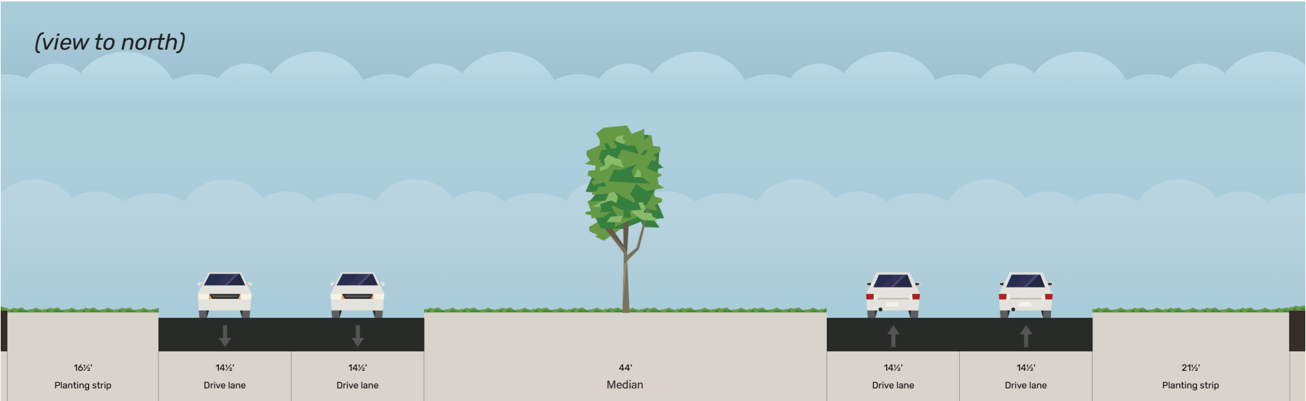
Exhibit 71. Typical Existing Cross-Section on FM 2499 (South of FM 2181) (140' ROW)
