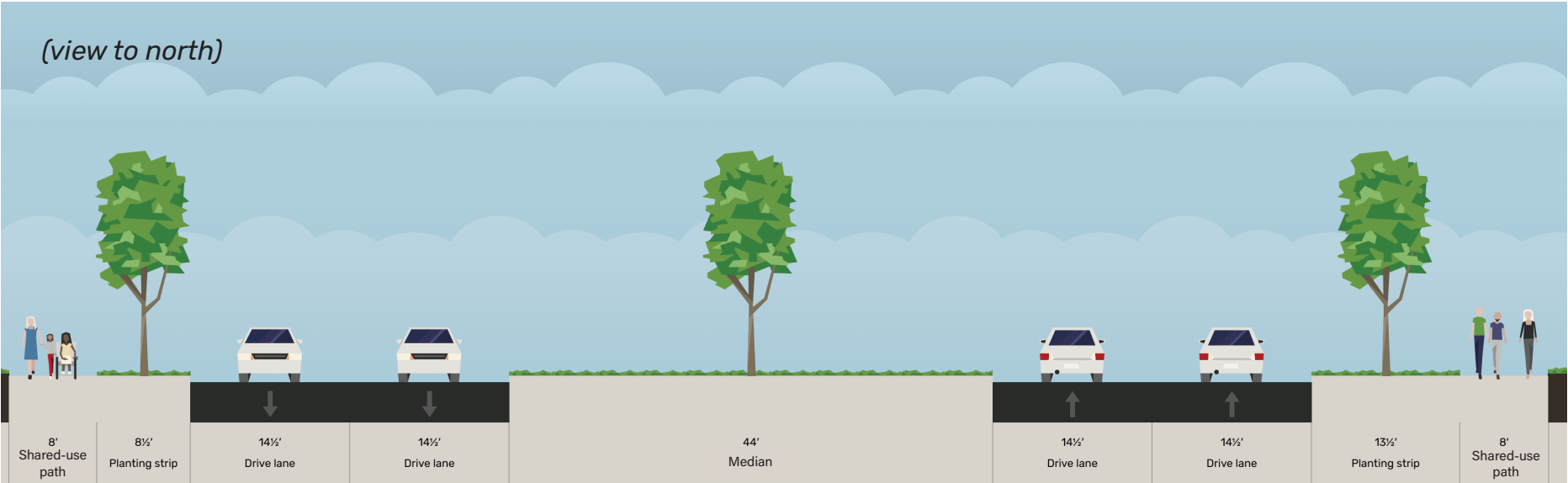
Exhibit 72. Proposed Typical Cross-Section on FM 2499 (South of FM 2181) (140' ROW)
